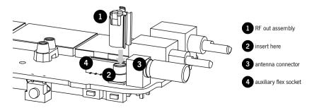
Figure D-11: Placing the RF out assembly (Orca Elan or Orca Excel shown)
