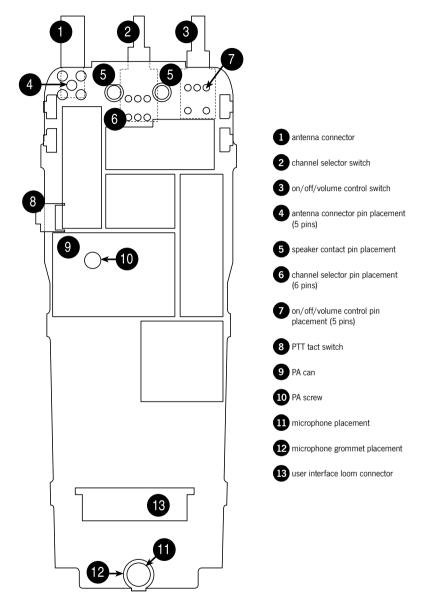
Figure D-9: Top surface of PCB, which is visible only when the PCB has been removed from the chassis (Orca Elan or Orca Excel shown)
